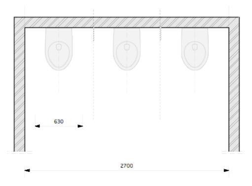
c. Now you mark the size of the front pilaster 270 mm on the floor and draw a line (see the illustration below) Why 270 mm? This is because we use the largest size of the door + margin (see detailed illustration).
