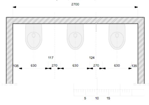
g. Mark door size + margin again (630 mm) and draw another line. You should have left at least +/- 135 mm from this last line to the right wall. If this is less, no panic, we can always cut this pilaster if needed (see the illustration above).
